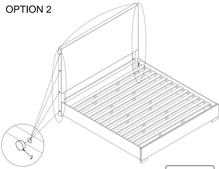
If not using wings, assemble the wood covers into the boreholes as shown in the instruction photo.
