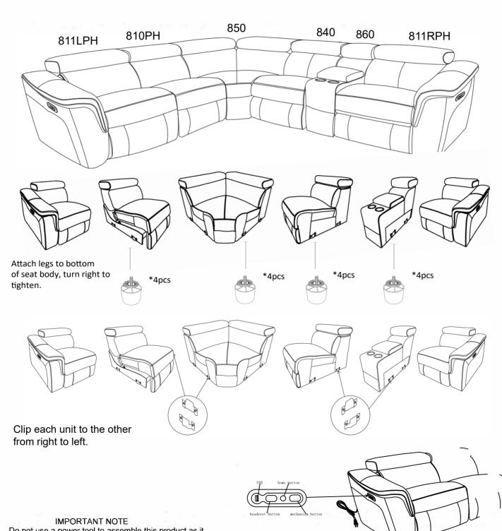
Do not use a power tool to assemble this product as it could damage the thread of the hardware and affect the solidity/durability of the product
