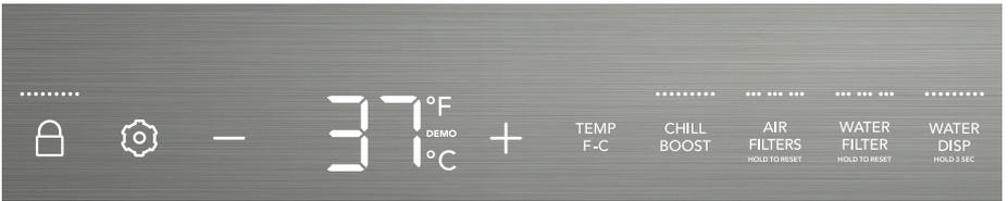
In the Sabbath mode, the **HIGH TEMP** alarm is active for health reasons. For example, if you leave the door ajar, the **HIGH TEMP** alarm is activated. The refrigerator will function normally once you close the door, without any violation of the Sabbath/holidays. The **HIGH TEMP** alarm comes on when the cabinet temperature is outside the safe zone for 20 minutes. The alarm silences itself after 10 minutes while the **HIGH TEMP** icon stays lit until you exit the Sabbath mode.
