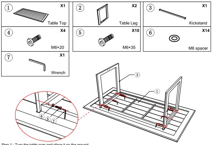
Step 1: Turn the table over and place it on the ground where the exterior finish will not be scratched.
