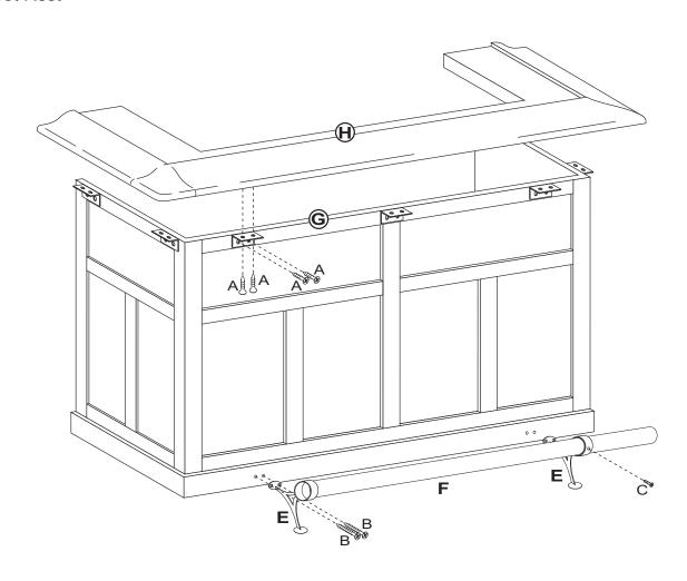
Begin assembly by attaching the Bar Top (H) to the Bar (G) by attaching each Metal Bracket (D) to the Bar (G) using 2 Wood Screws (A) per each bracket. Once secured, rest Bar Top in place and secure using also 2 Wood Screws (A) to hold in place. Tighten all screws only using a phillips head screwdriver (not included).
