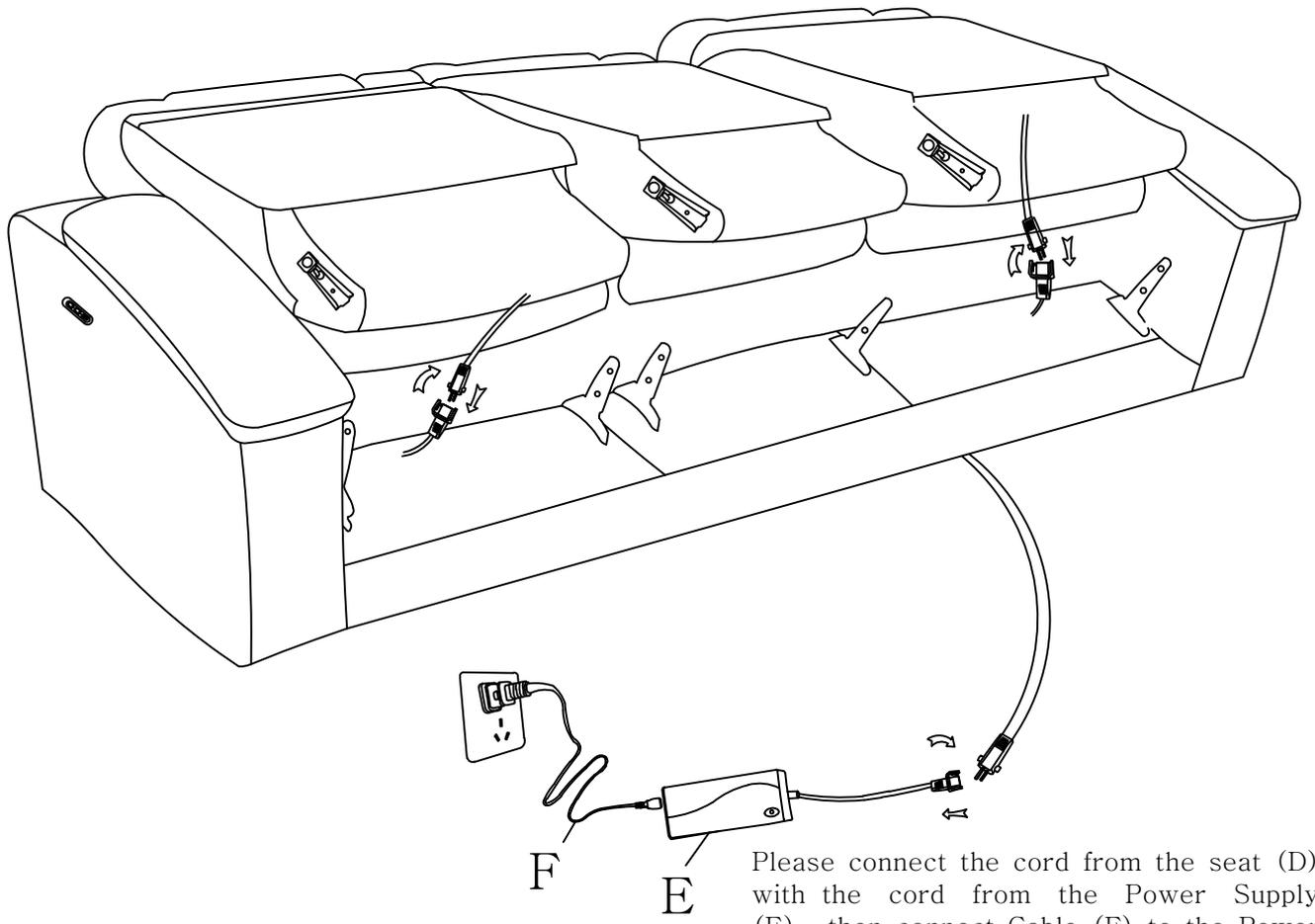
Please connect the cord from the seat (D) with the cord from the Power Supply (E), then connect Cable (F) to the Power Supply (E).
