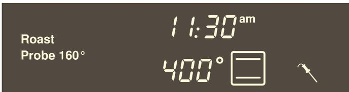
5. Set the internal temperature for the probe; for instance, press 1 4 5 to set the probe temperature to 145°. See cooking charts for appropriate internal temperatures. The adjusted probe temperature appears in the display:
