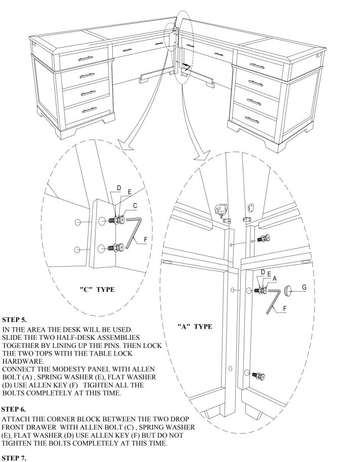
WITH ALL THE ALLEN BOLTS STARTED YOU CAN TIGHTEN ALL THE ALLEN BOLTS PULLING THE ASSEMBLIES TIGHT AND INTO THE CORRECT FIT. COVER THE BOLTS WITH COVER CAPS (G).
