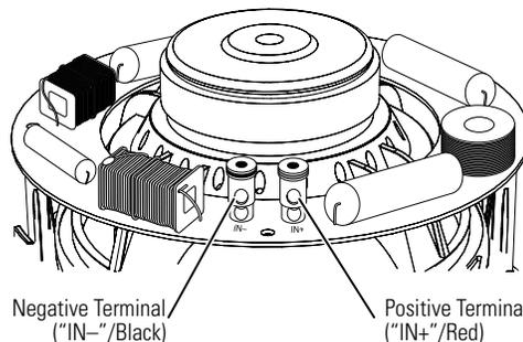
Press down on the top of the terminal to open the hole; insert the bare end of the wire into the hole; and release the terminal to secure the wire.
