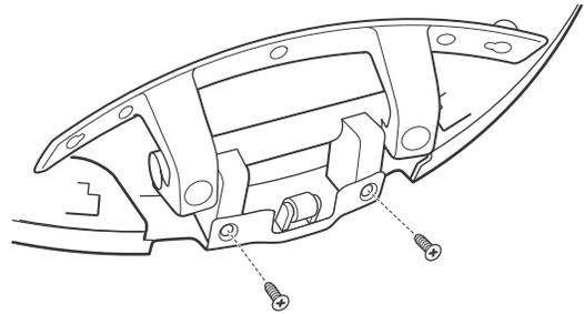
13. Hold the door on its side with one hand and fasten the remaining 2 screws as shown. Then tighten the 2 screws (#8) holding the hinge assembly.
