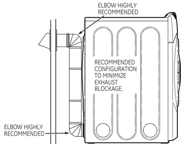
**NOTE: ELBOWS WILL PREVENT DUCT KINKING AND COLLAPSING.**
