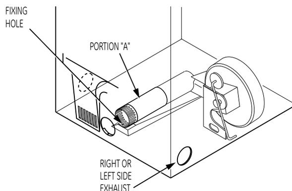
Reconnect the cut portion (A) of the duct to the blower housing. Make sure that the fixing hole is aligned with the tab in the base. Use the screw saved previously to secure the duct in place through the tab on the appliance base.
