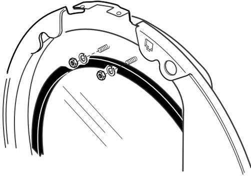
15. Place the hinge cover in position. Align the hinge cover holes with the holes in the door.
