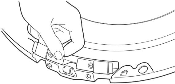
16. Secure the hinge cover with the 2 tapping screws (#8).
