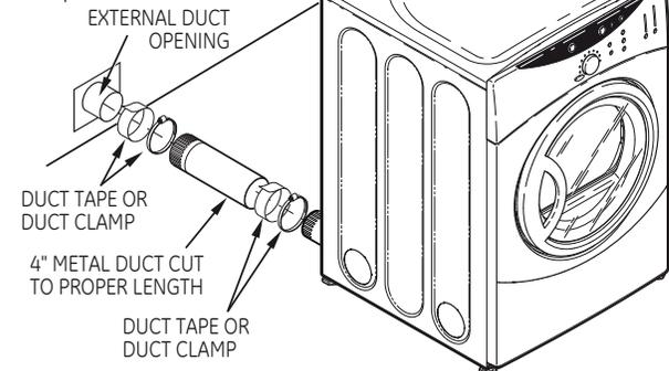
**NOTE: WE STRONGLY RECOMMEND SOLID METAL EXHAUST DUCTING. HOWEVER, IF FLEXIBLE DUCTING IS USED IT MUST BE UL-LISTED METAL, NOT PLASTIC.**
