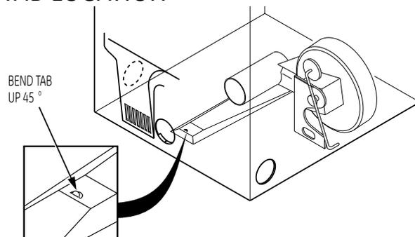
Through the rear opening, locate the tab in the middle of the appliance base. Lift the tab to about 45° using a flat blade screwdriver.
