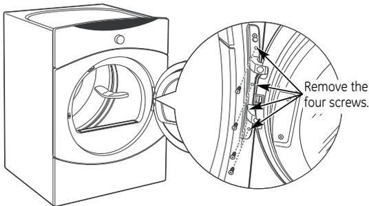
3. Loosen the top screw as shown. Unhook the door by lifting and pulling as shown by the arrows.
