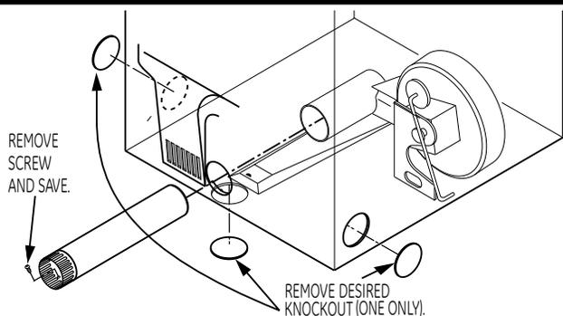
Detach and remove the bottom, right or left side knockout as desired. Remove the screw inside the dryer exhaust duct and save. Pull the duct out of the dryer.
