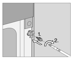
■ Insert the bolt into the mounting aid and tighten it in the cabinet niche.
