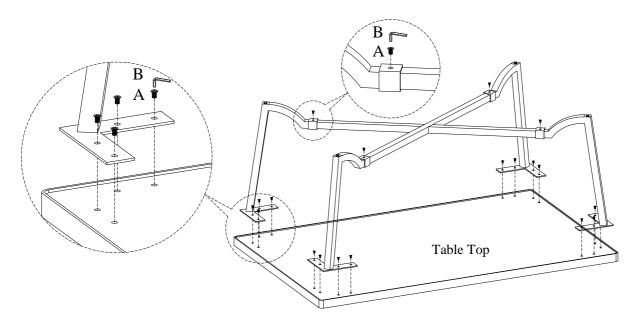
STEP 2: Put the table top face down on a soft surface, Attach the legs with X stretcher to the table top by using 20 bolts(A). Completely tighten all bolts. Turn the assembled table to the upright position.
