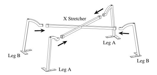
STEP 1: Insert the legs A and legs B to the X stretcher as shown.
