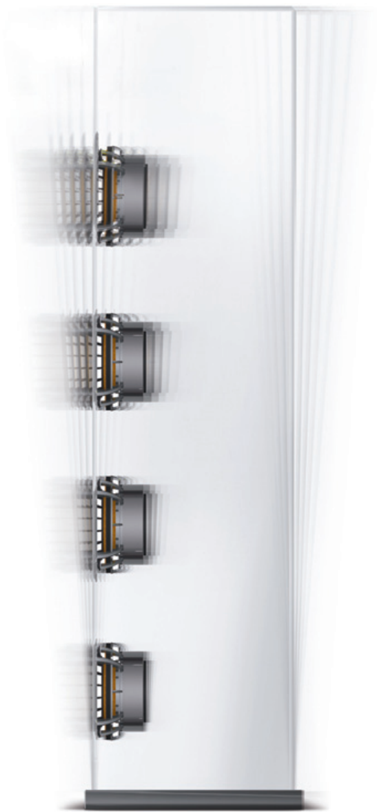
Conventional speaker generating cabinet resonance
