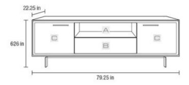
Open Center Compartment Interior Dimensions (H x W x D) 7.75 x 33.5 x 17.5 in **Fixed Shelf Capacity** Center Component Compartment Interior Dimensions (H x W x D) 7.5 x 32 x 17.5 in **Bottom Shelf Capacity** 100 lbs Side Component Compartment Interior Dimensions (H x W x D) 16 x 19.5 x 20.5 in Adjustable Shelf Capacity 50 lbs **Bottom Shelf Capacity** 100 lbs
