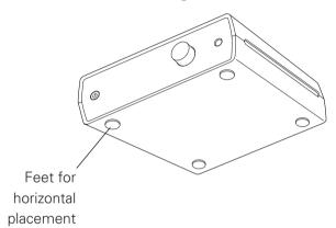
Attach the feet for horizontal placement as shown in the figure.
