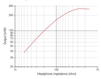
• 1x 3.5mm phone jack: maximum output 3V rms off load, THD below 0.002%, output impedance  $2.2\Omega$ , short-circuit protected.
