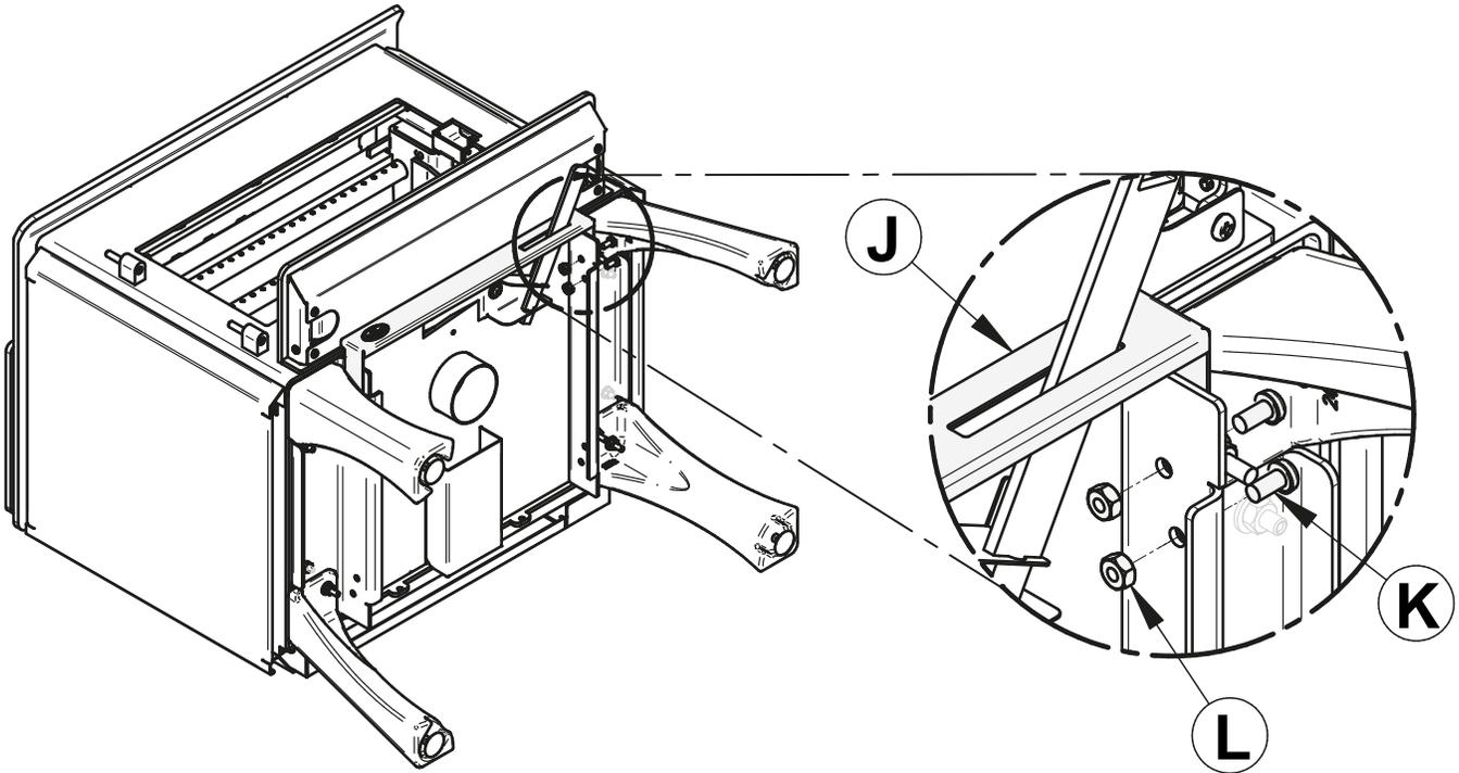
6. Put the stove on its legs, install the ash drawer included with the kit. Put back the firebricks, the ash plug and the door on the stove. See step 1.
