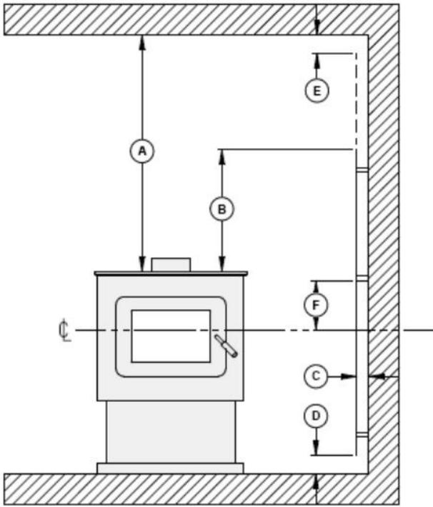
Figure 24: Heat shield clearances
