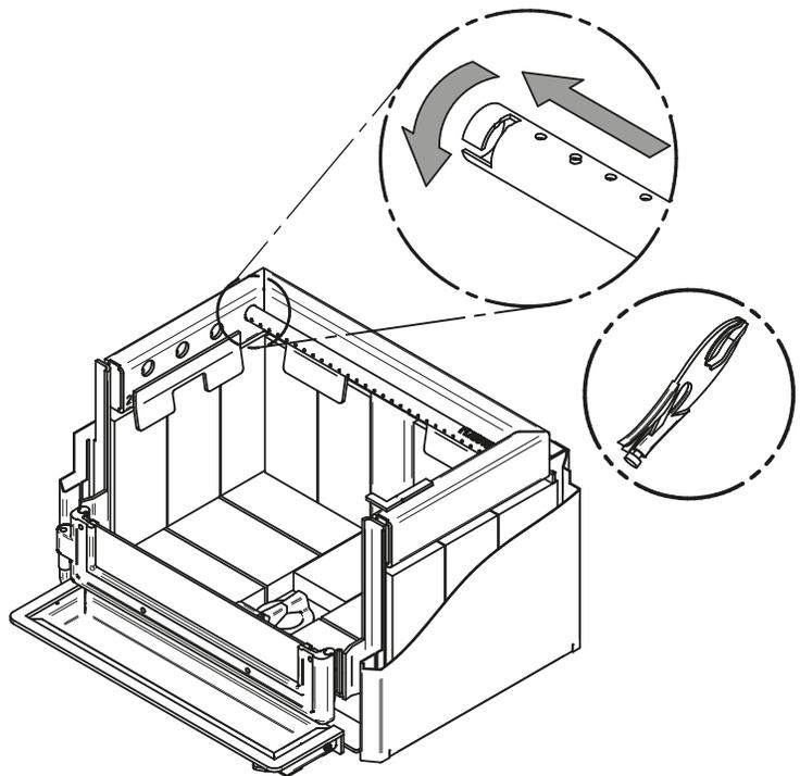
Note that secondary air tubes (B) can be replaced without removing the baffle board (A) and that all tubes are identical.
