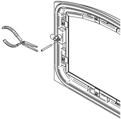
Figure 17: Removing the split pin
