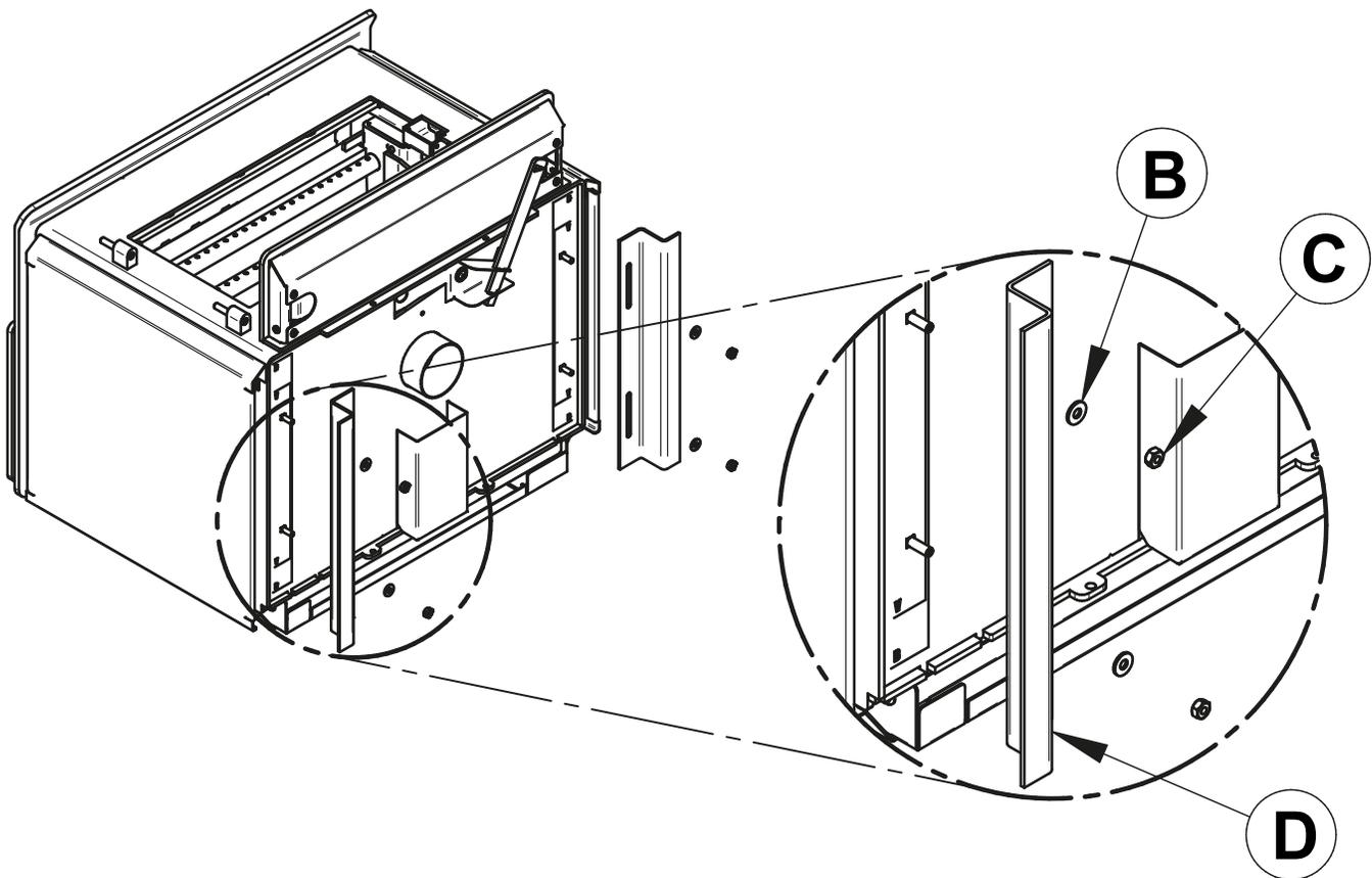
3. Install the pedestal **(E)** on the stove and screw it in place using washers **(B)** and nuts **(C)**.
