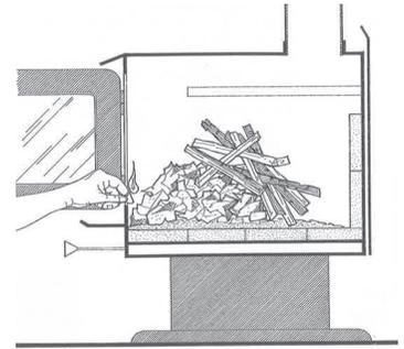
Once the fire has ignited, the door can be closed with the air control still fully open. When the kindling is almost completely burned, standard firewood pieces can be added.
