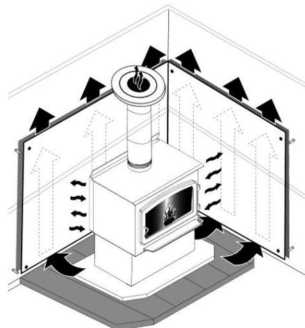
Figure 23: Heat shield
