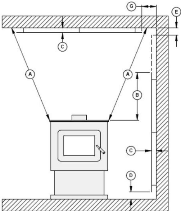
Figure 26: Heat shield clearances
