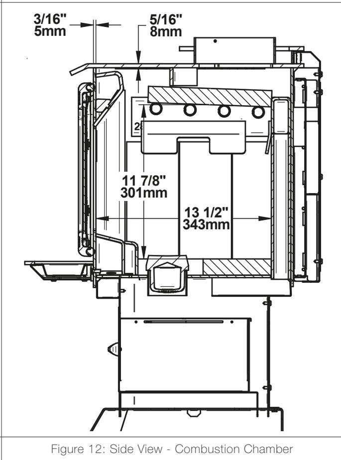
Figure 12: Side View - Combustion Chamber
