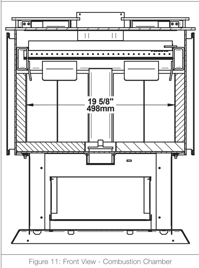
Figure 11: Front View - Combustion Chamber
