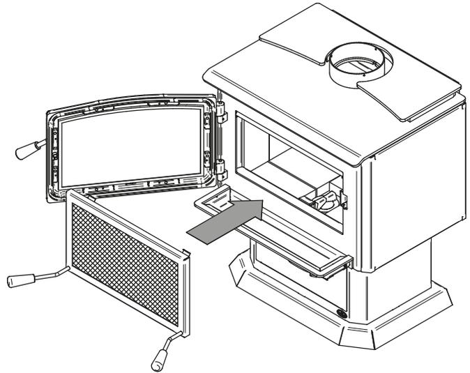
3. Lean the upper part of the fire screen against the top door opening making sure to shove the top fire screen brackets behind the primary air deflector.
