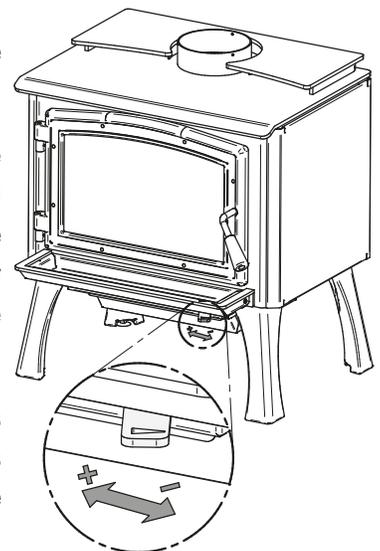
On the other hand, too much air can make the fire uncontrollable, creating very high temperatures in the unit as well as in the chimney and seriously damaging them. A reddish glow on the unit and on the chimney components indicates overheating. Excessive temperatures can cause a chimney fire.
