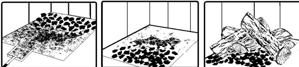
Raking the coals is useful for two reasons. First, it brings them near where most of the combustion air enters the firebox. This will ignite the new load quickly. Secondly, the charcoal will not be smothered by the new load of wood. When the embers are simply spread inside the combustion chamber, the new load smoulder for a long time before igniting.
