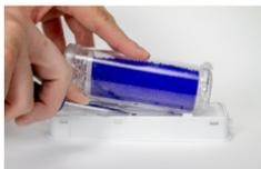
4. Install a new cartridge filled with blue beads on the Desiccant Dryer Door.
