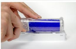
3. Continue holding the Locking Tab down and slide the Desiccant Dryer Cartridge upwards to remove it from the Desiccant Dryer Door.
