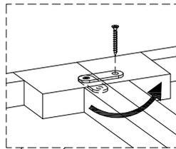
**STEP 1:** Take off one screw from each mounting plate and swing it to the proper location on the other bookcase before re-securing it with the screw.
