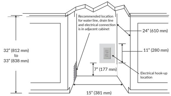
NOTE: For Gravity drain models, the drain hole cannot exceed 7 inches above the floor. For Pump models, the drain hole should be no lower than 7 inches and no higher than 4 feet above the floor.
