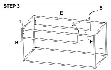
Step 3: Attach Shelf Frame (F) to LSF Leg Frame (B) and Table Base Rail (E) using Small Bolt (1) and Long Bolt (3) as shown. Tigthen with an Allen Key (5).
