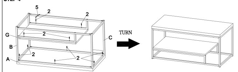
Step 4: Place Table Top (A) on a soft and clean surface to prevent finish from scratching. Place the table assembly in Step 3 onto Table Top (A). Insert Medium Bolt (2) into the holes of Table Top Side Rail (D) and LSF/RSF Leg Frame (B,C), and secure with an Allen Key (5).
