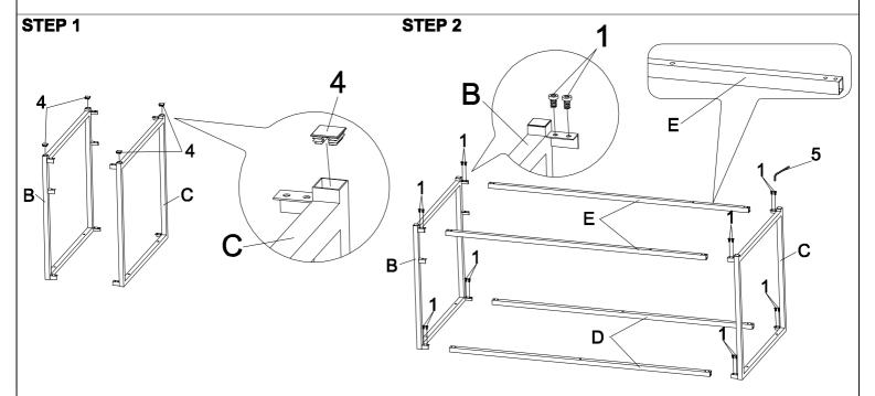
Step 1: Insert Cap (4) into LSF/RSF Leg Frame (B,C) as shown.
