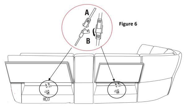
**STEP 7**: Connect the power cords of all power recliners (released in **Step 2**) to each others. Make sure to close the clip lock to prevent the connection from coming loose. Extra cores are used when change the order of furniture. (See the Figure 7.)
