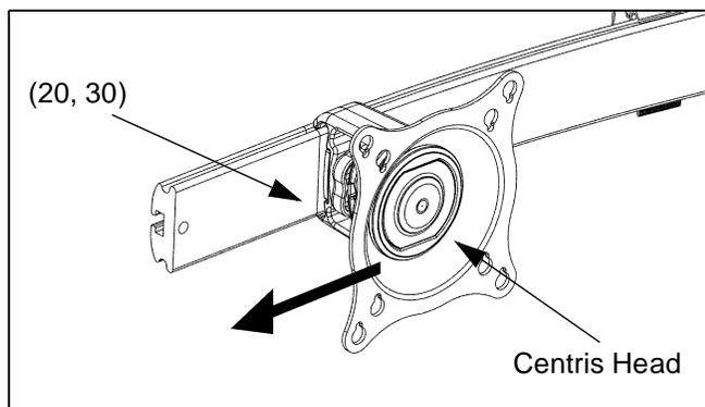
**Figure 9: Slide Centris Bracket off Array Rail**
