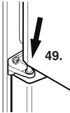
**49.** Suspend top door on hinge pin. For this, the door must be open at least 90°.
