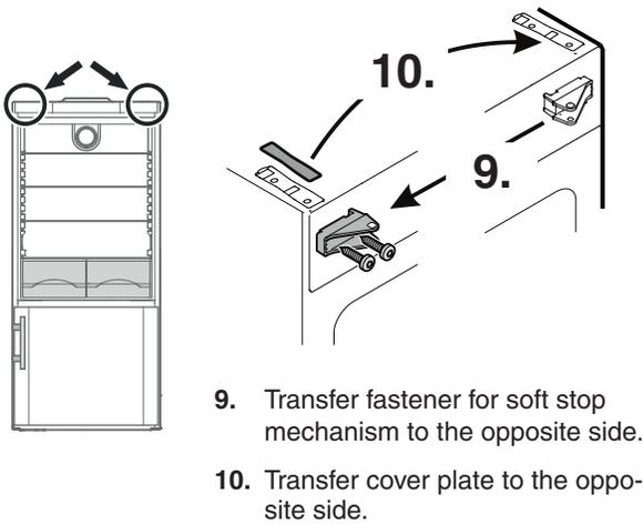
9. Transfer fastener for soft stop mechanism to the opposite side.
