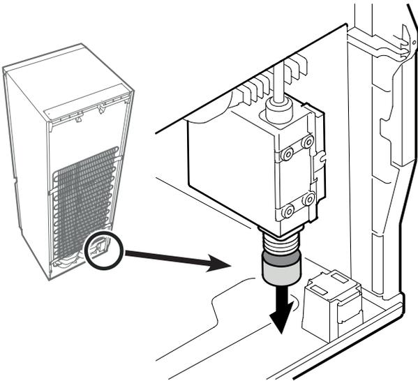
3. Connect the water line to the adapter in the respective configuration, depending on the type of water line used.
