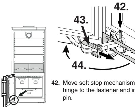
42. Move soft stop mechanism hinge to the fastener and insert pin.
