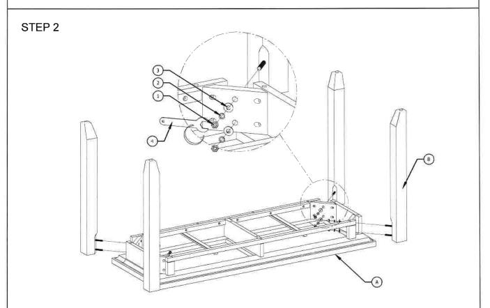
Step 2: Attach leg(B) into the top table(A). insert the hexagonal nut(1), lock washer (2), flat washer (3) into bolt, tighten with wrench(4).
