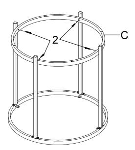
Step 2: Attach Bottom Frame (C) to the table assembly in Step 1 using Long Bolt (2) as shown.
