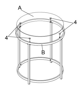
Step 3: 1.Insert Suction Cup (4) onto Top Frame (B) as shown. 2.Place the Glass (A) to the Suction Cup (4) as shown.
