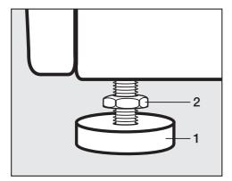
■ Using the wrench supplied, turn counter nut 2 in a clockwise direction. Then turn counter nut 2 together with foot 1 to unscrew.
