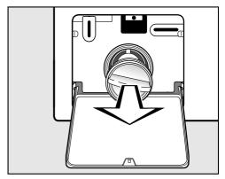
■ Remove the drain filter completely.
