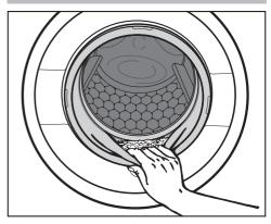
Check the folds in the door seal for any small articles.
