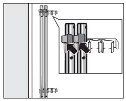
■ Secure the shipping struts to the back of the washing machine. Make sure the top catch is located above the holder.
