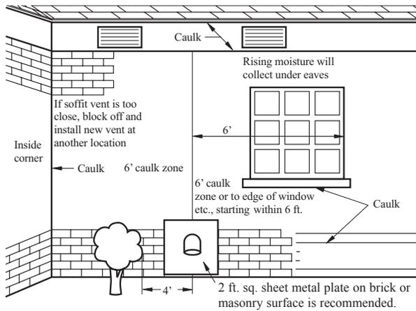
**⚠ WARNING:** Moisture in the flue gas will condense as it leaves the vent terminal. In cold weather this condensate can freeze on the exterior wall, under the eaves and on surrounding objects. Some discoloration to the exterior of the building is to be expected. However, improper location or installation can result in severe damage to the structure or exterior finish of the building
