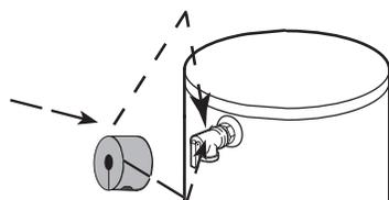
Typical Side Connect T & P Arrangement.
