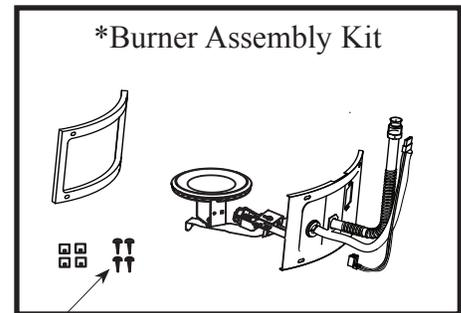
The kit provides extra speed clips and tamper resistant screws.
