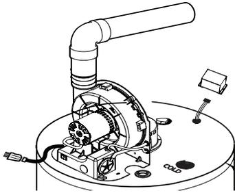
13. The User Display will be mounted to the plastic Water Heater Mounting Bracket.
