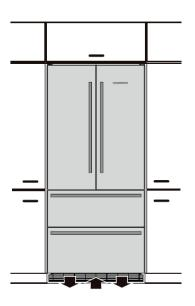
CBS 20 appliances don't need any ventilation openings in the cabinet. The required airfl ow is directed through the toe kick area.
