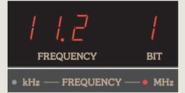
Sampling frequency and quantization bit display
