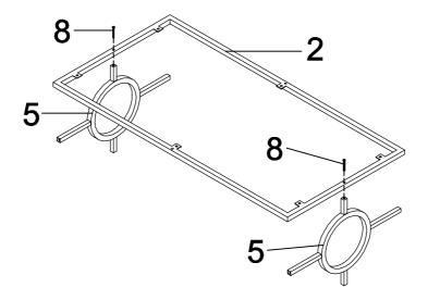
Step 1: Attach Small Frame (5) to Top Frame (2) using Long Bolt (8) as shown.
