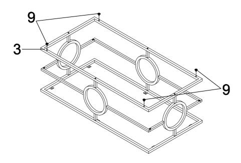
Step 4: Insert Leveler (9) onto Bottom Frame (3) as shown.
