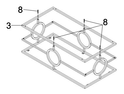
Step 3: Attach Bottom Frame (3) to the assemble in Step 2 using Long Bolt (8) as shown.
