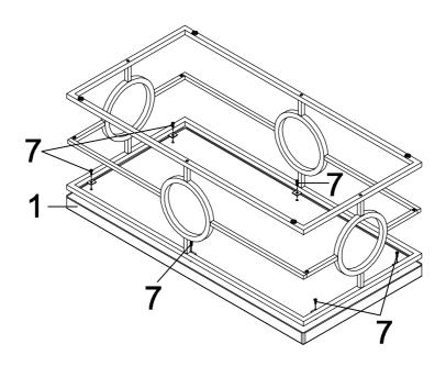
Step 5: Attach the assemble in Step 4 to Mirror Box (1) using Medium Bolt (7) as shown.
