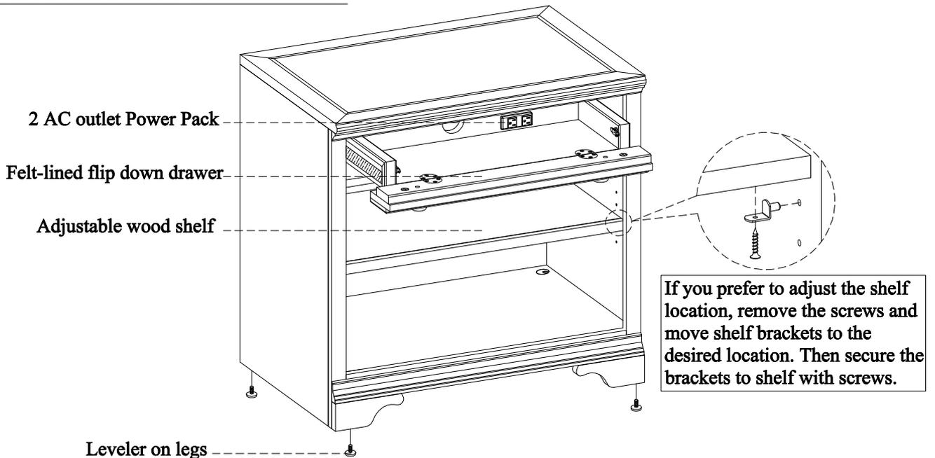
Adjust the leveler when necessary
