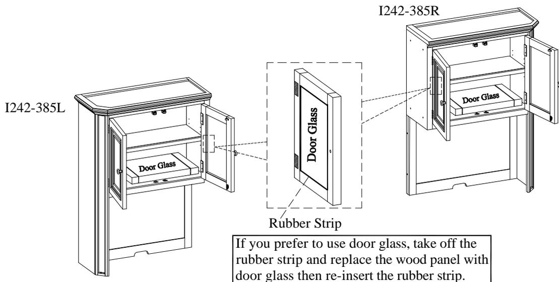
If you prefer to use door glass, take off the rubber strip and replace the wood panel with door glass then re-insert the rubber strip.
