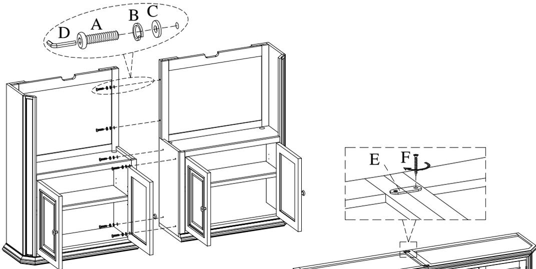
**STEP 2:** Return the assembled hutch to the right side up position. Attach the mounting plates (E) to assembled hutch as shown right by using 4 screws (F).
