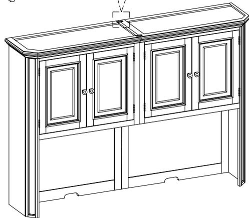
**STEP 3:** Put the assembled hutch on the assembly desk. Take off one screw from each metal plate on the back of hutch and swing it in an ideal place. Then re-secure the metal plate with screw to assembly desk.
