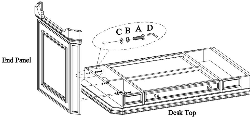
**STEP 2:** Remove the fake drawer front on the desk base of -338. Align the hole in the front rail of desk base with the insert in the end brace of desk top. Attach the desk top with end panel to the desk base using 3 bolts(A), lock washers(B) flat washers(C) and wood screws (E).
