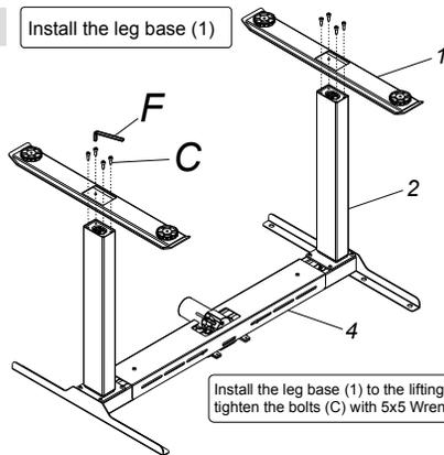
Install the leg base (1) to the lifting leg (2), and tighten the bolts (C) with 5x5 Wrench (F).
