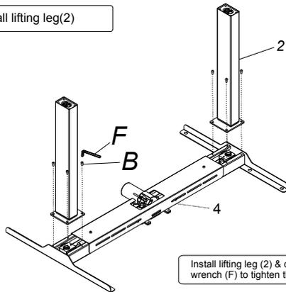
Install lifting leg (2) & crossbeam (4) together, use 4\*4 wrench (F) to tighten the bolts (B).
