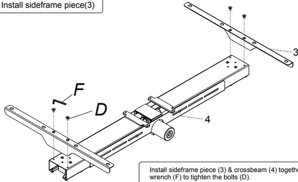
Install sideframe piece (3) & crossbeam (4) together, use 4\*4 wrench (F) to tighten the bolts (D).
