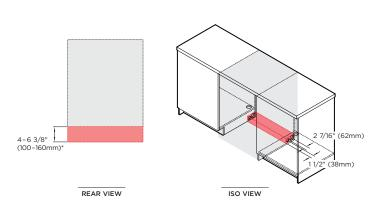
Service outlet at rear extends both sides, hoses and cords can be routed to either or both sides. \*Depending on adjustment of levelling feet.
