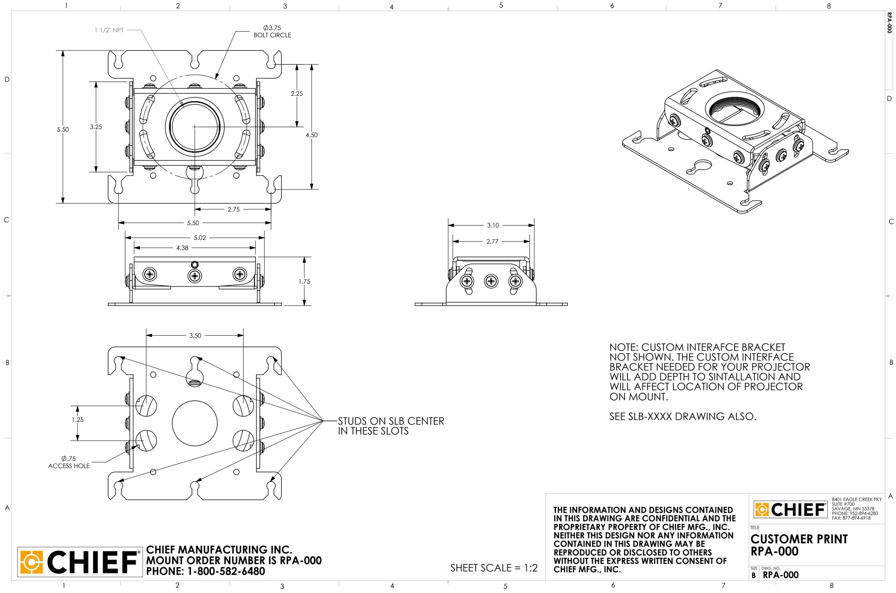
NOTE: CUSTOM INTERAFCE BRACKET NOT SHOWN. THE CUSTOM INTERFACE BRACKET NEEDED FOR YOUR PROJECTOR WILL ADD DEPTH TO SINTALLATION AND WILL AFFECT LOCATION OF PROJECTOR ON MOUNT.
