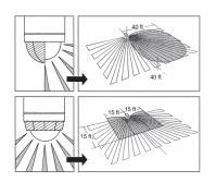
Shrouds, supplied with each unit, snap in place, allowing users to adjust coverage as needed.
