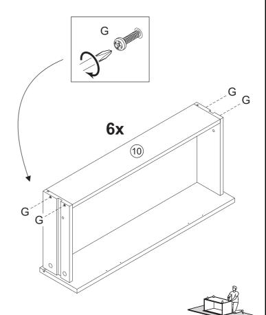
Insert parts 9 and 10 between parts 5, 6 and 7. Secure part 10 with screw (G) and phillips screwdriver.
