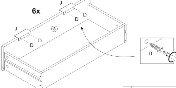
Secure handle (J) with screw (D) and phillips screwdriver, in the pre-drilled holes on the drawer front 8.
