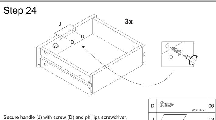
in the pre-drilled holes on the drawer front 23.
