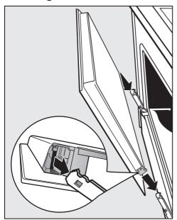
Hold the door securely on both sides and carefully install it back into the hinge retainers.
