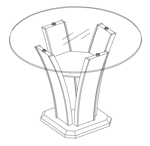
Do not tighten screws until completely assembled.
