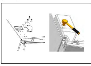
11. Install the PCB in the door hinge cover
