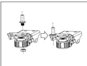
4. Unscrew the left adjustable leveling foot and loosen the screw.
