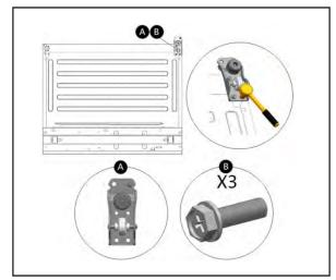
3. Unscrew and insert the hinge pin on the opposite side of the bottom hinge using an adjustable wrench and pliers.
