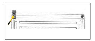
8a. Using an 8 mm socket with a ratchet: Unscrew right top hinge cover and left top decorative cover, and disconnect the door switch and display.
