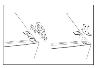
9. Remove the front top decorative doorcover, turn the cover (together with the connecting wire) 180° and install it.
