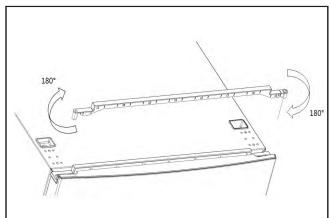
10. Install the top left hinge (provided in the spare parts bag).
