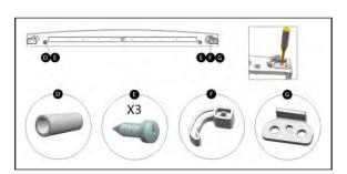
6. Reinstall the aid-closer (F), metal block (G) onto the left side, and the supporter (D) onto the right side.
