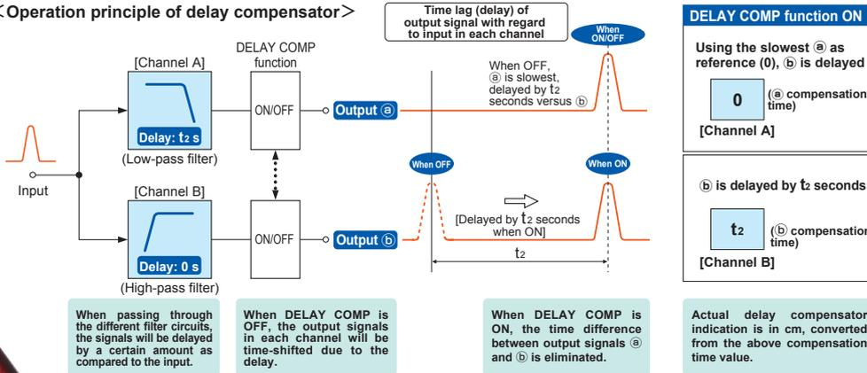
When a signal passes a filter circuit, a delay necessarily occurs. The "DELAY COMP" function compensates for such delays. The illustration at left uses a 2-way system as an example to show how the delay compensator works.
