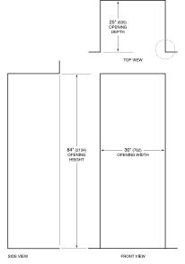
IOTE:  $3^{1}/2^{*}$  (89) finished returns will be visible and should be finished to match cabinetry.
