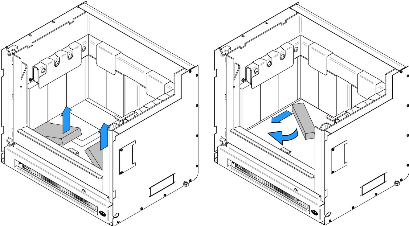
3. Remove the back bricks (4), then remove the back left brick (1).
