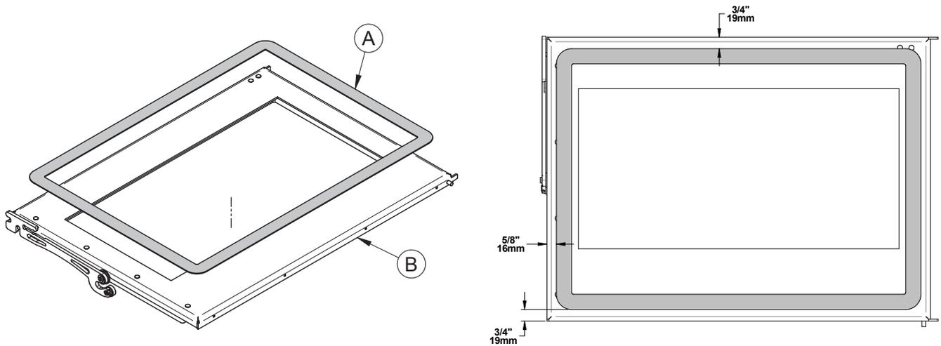
Figure 15: Replacing the glass gasket on the door
