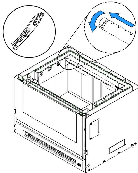
3. Repeat steps 1 and 2 for the two tubes in the back then *install the baffle before installing the two front tubes.*
