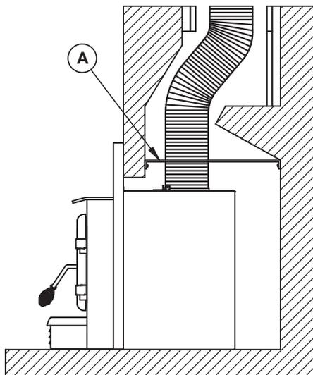
Figure 27: Block-off Plate
