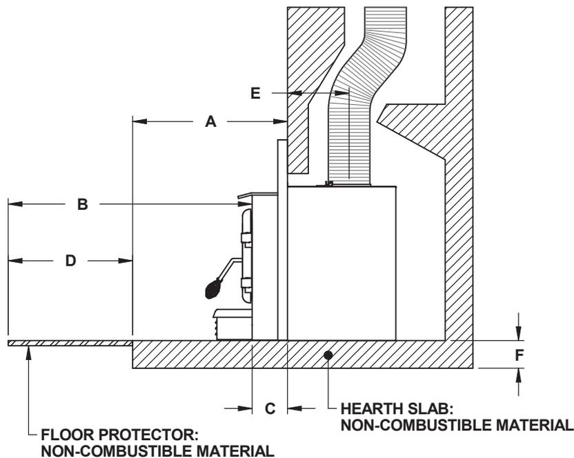
Figure 24: 5" or less raised base installation
