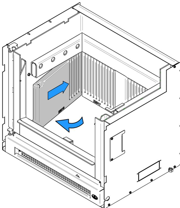
7. Install the refractory slab retainer (2) on both sides and screw them in place .
