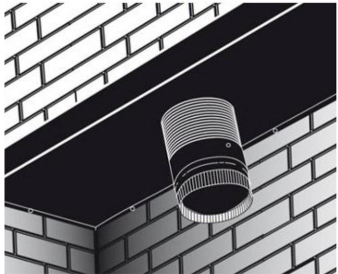
Figure 28: Block-off Plate
