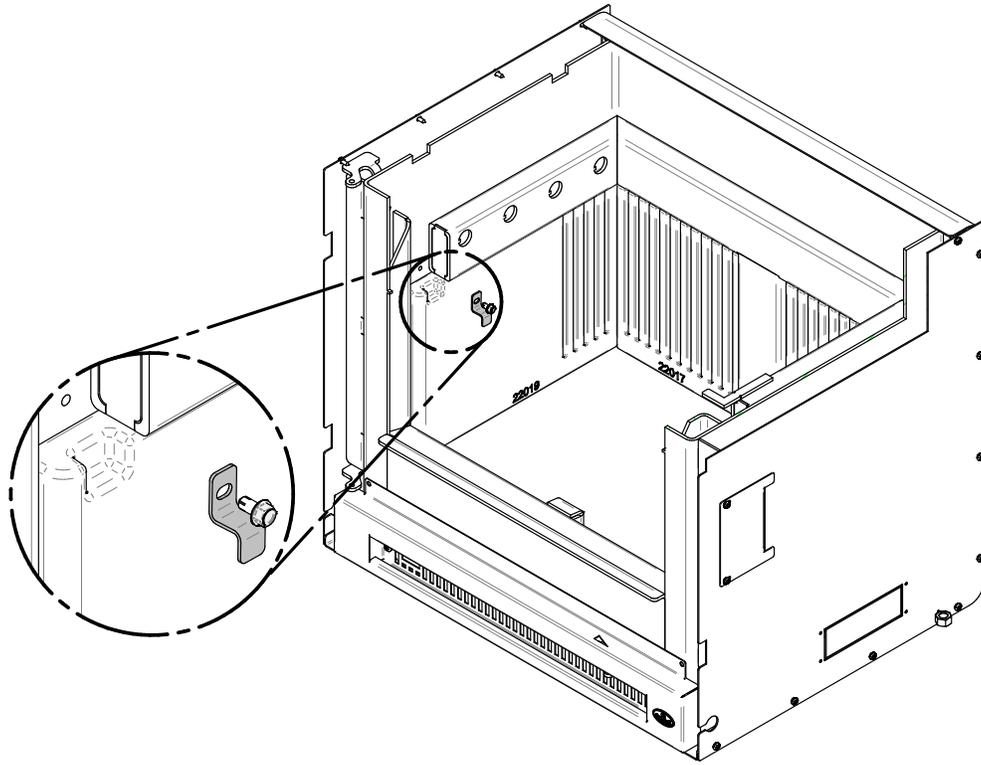
8. Install the floor refractory slabs.
