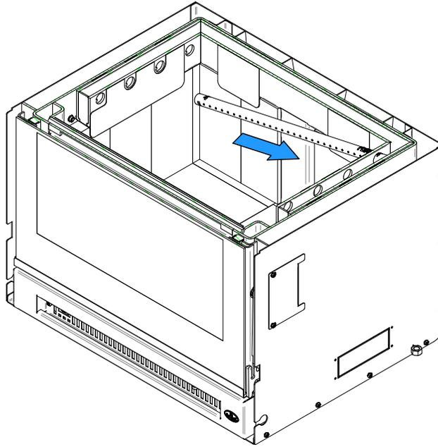
2. Align the notch in the left end of the tube with the key of the left air channel hole. Using a « Wise grip » hold the tube and lock it in place by turning the tube. Make sure the notch reaches the end of the key way.
