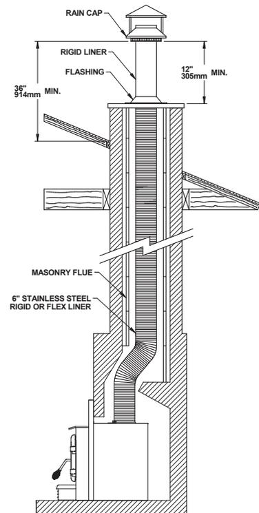
Figure 29: Liner Installation
