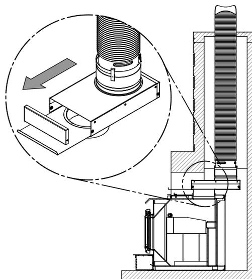
Figure 33: Offset liner adaptor
