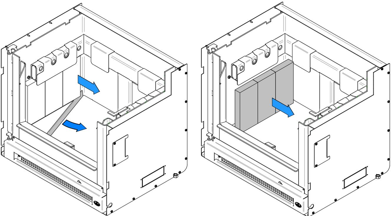
5. Remove the retainers (4) and install the back refractory bricks (2). The retainers cannot be reused after being removed so they can be disposed of.
