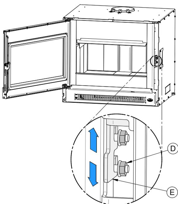
4. Unscrew the nuts **(D)** and lift the door latch mechanism **(E)** to increase the pressure on the door. Lower the mechanism **(E)** to release pressure.
