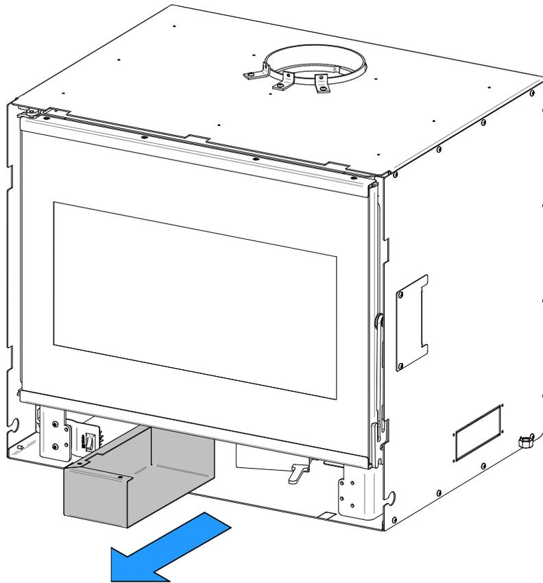
5. Remove both wing nuts **(A)** holding the blower mounting plate.
