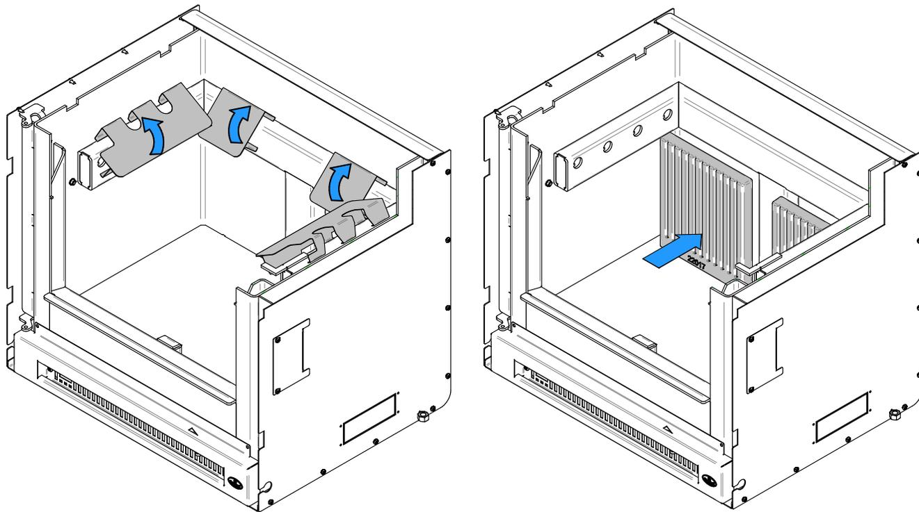
6. Install the sides (2) refractory slabs.
