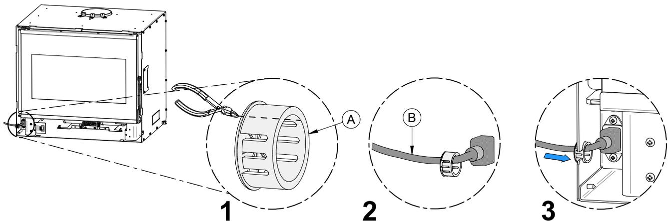
Figure 7: Plugging in the blower power cord
