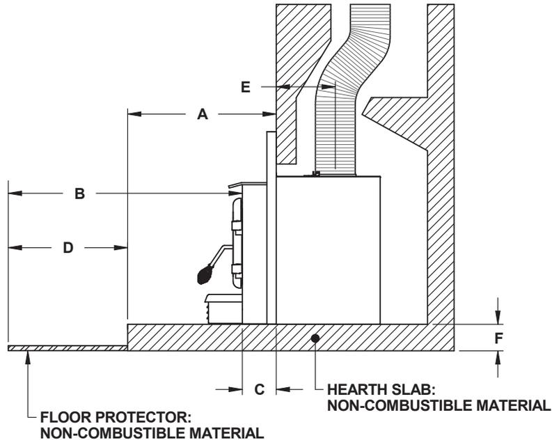
Figure 25: More than 5" raised base installation
