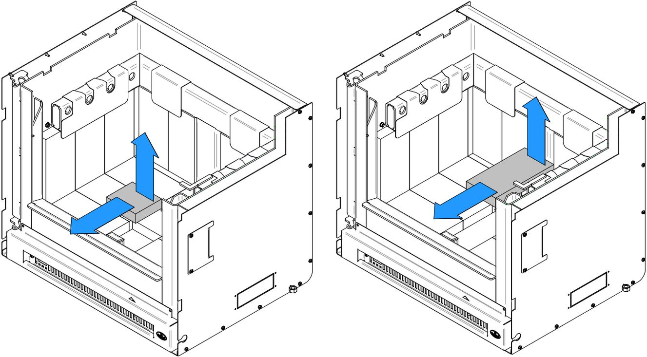
2. Remove the other floor bricks (6). Then, remove the back bottom bricks (2).
