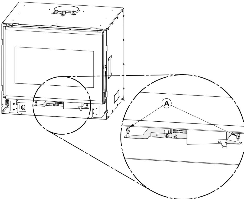
6. Rotate the blower counterclockwise and gently pull on the blower.
