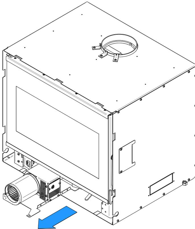
7. Remove both screws **(B)** and gently pull on the plate **(A)**. Unplug the blower wires **(C)**. Once the blower is unplugged, pull gently for removal.
