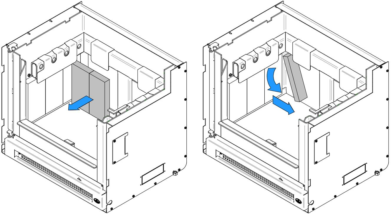
4. Remove the brick retainer (1) and the left bricks (3). Repeat on the right side.
