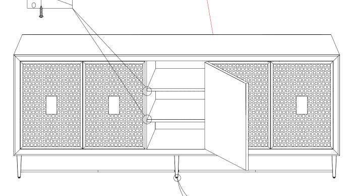
Adjust leveler if needed to level credenza on uneven floor.
