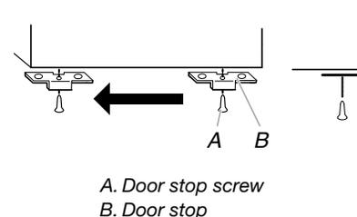
2. Replace the door stop on the opposite side of the refrigerator door, making sure that the hole in the door stop plate is aligned perfectly with the hole for the bottom hinge pin.
