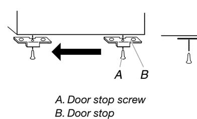
6. Move the door stop to the opposite side, making sure that the hole in the door stop plate is aligned perfectly with the hole for the center hinge pin.
