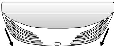
3. Remove the light bulb and replace it with an appliance bulb of the same size and shape.
