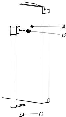
3. Using the plastic tool (provided), remove the brand badge from the freezer door by prying up the right-hand side and slowly peeling the badge away from the door, revealing the hole to mount the door handle.
