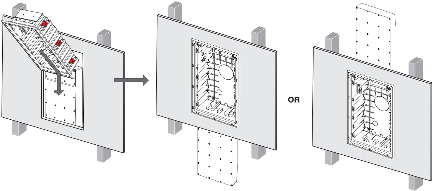
The reservoir box can be fitted within the wall either above or below the back box to enhance the speaker's low frequency performance. A clear distance within the wall should be reserved to accommodate the reservoir box.
