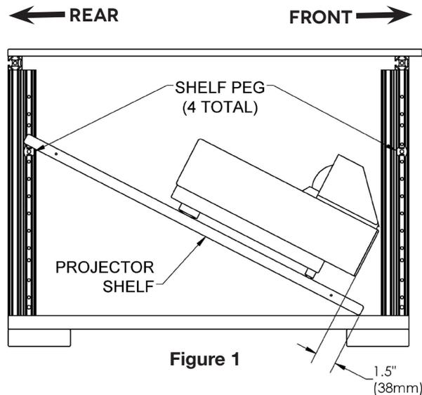
3. Continuing holding the back end of shelf, while a 2nd person lifts the shelf up and slightly forward until the projector lens housing goes through the opening in the top and the shelf can be rested on the front shelf peg as shown in figure 2.
