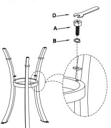
Step 3 All part was properly assembled, tighten up Hexagonal Bolt (A) at the Shelf with Wrench (D).
