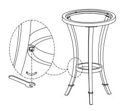
Attach the Top Metal Frame to the assembled base using the Hexagonal Bolts (A), Lock washer (B), Flat washer (C) and tighten with Wrench (D),
