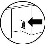
TIP: IN TIGHT INSTALLATIONS CUT THROUGH AN ADJACENT CABINET WALL TO REACH AN OUTLET INSTALLED THERE
