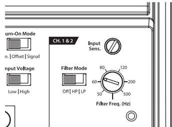
1) “**Filter Mode**” Control: The XD200/2v2 employs a 12dB per octave filter which can be controlled or defeated completely by way of the three-position “Filter Mode” switch:
