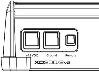
The XD200/2v2's “+12 VDC” and “Ground” connections are designed to accept 8-4 AWG power wire. **8 AWG is the minimum required wire size for this amplifier.**
