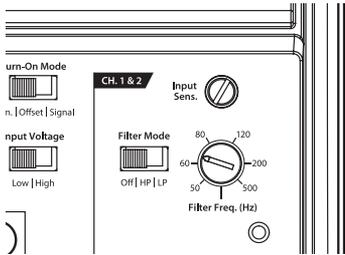
To properly set the amplifier for maximum clean output, please refer to Appendix A (page 12) in this manual. After using this procedure, you can then adjust the “**Input Sens.**” levels downward if this is required to achieve the desired system balance.
